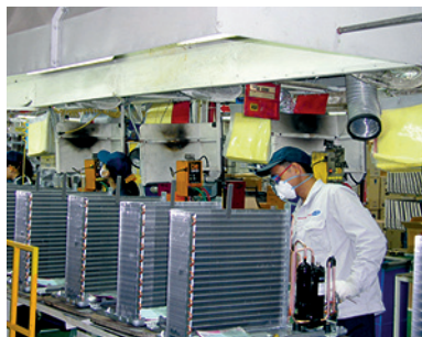
Outdoor units production
